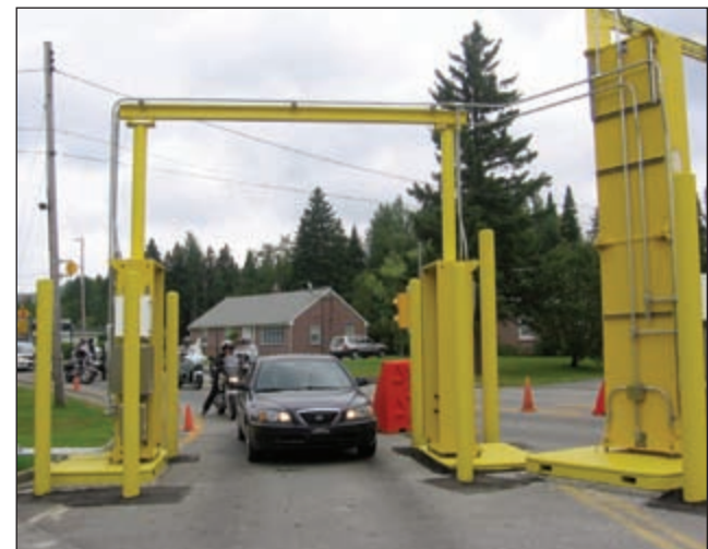
Cars crossing the United States border at Coburn Gore enter a new radiation portal monitor. The non-intrusive machine, in place by September, detects both legitimate and illegitimate radiation and is one of 374 located at borders across the U.S.
